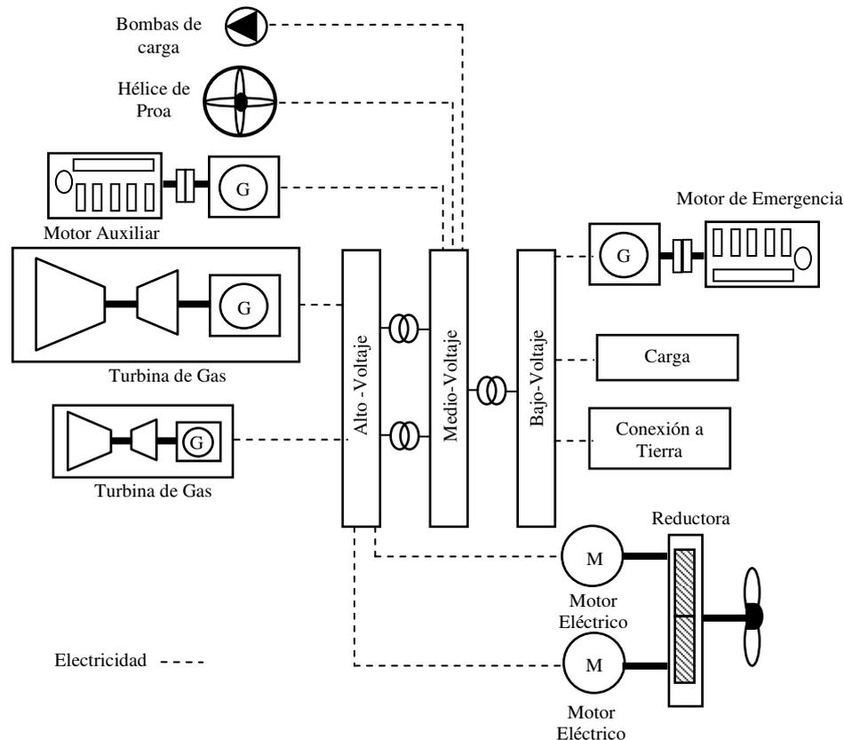
**Fig. 2.6.** DFGE (dual-fuel gas turbine electric propulsion).
