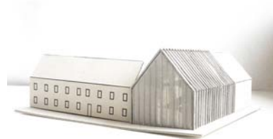
> the west facade is covered with concrete pillars and an inner translucent skin
