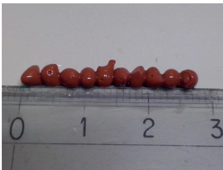
Figure 8.5. Image of the chitosan red mud beads.
