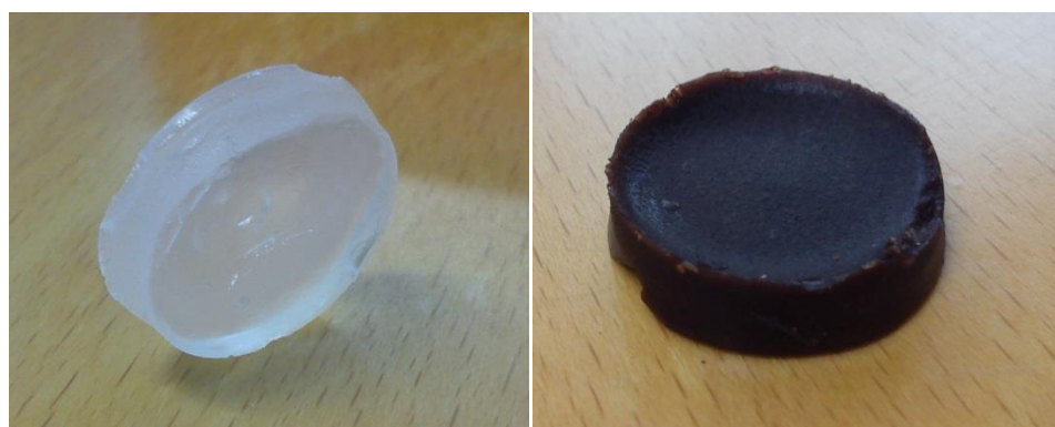
Figure 7.1. Pictures of the blank gel (left) and fern-containing gel (right) composite pellets. Pellet dimensions are 2.3 cm diameter and 0.5 cm height.
