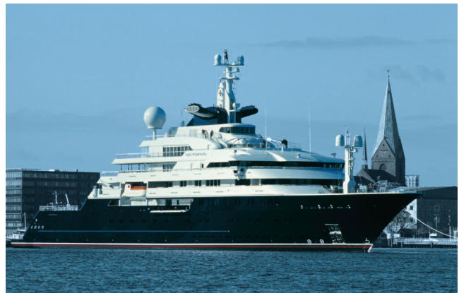
126 M MEGAYACHT OCTOPUS Manoeuvring aid: 2 x STT 330 TLK (350 kW each) 1 x SCHOTTEL Rudderpropeller Type SRP 330 ZSV (450 kW)
