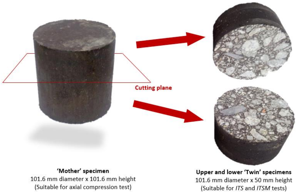
Figure 3. Schematic process to obtain two 50 mm height 'twin' specimens from the same 101.6 mm height 'mother specimen'. Three specimens have exactly the same intrinsic properties (specific gravity, voids content, moisture content, etc)
