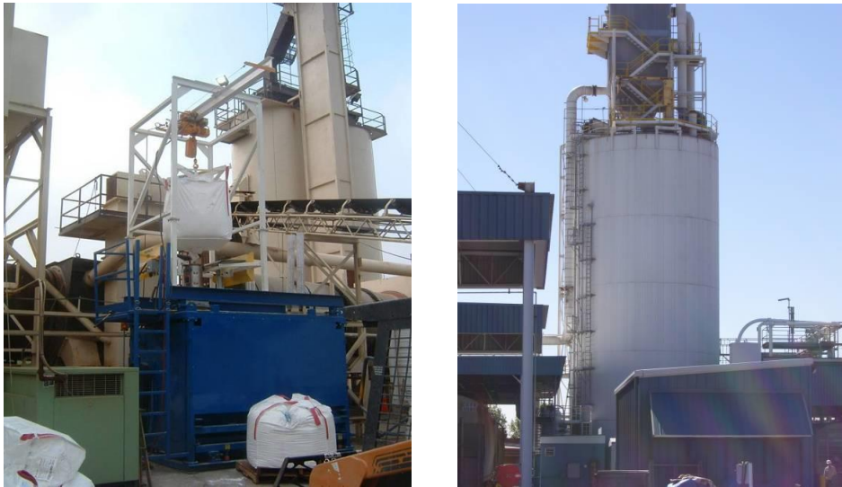
Fig.5. Feeder filling with machinery that can unload bulk bags or through a connection to a silo [3].
