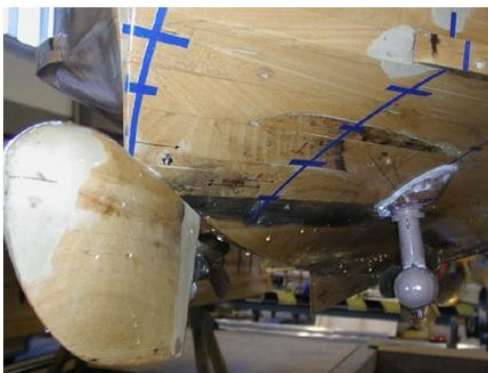
Figure 7: Illustration of "bulb" fin
