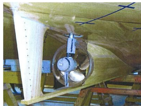
Figure 4: Single ducted thruster unit arrangement
