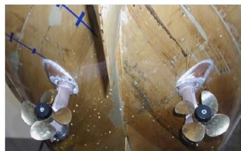
Figure 6: Twin (wing) thruster units arrangement
