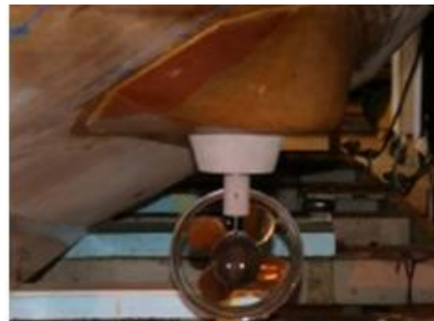
Figure 9: Thruster head box with additional cone
