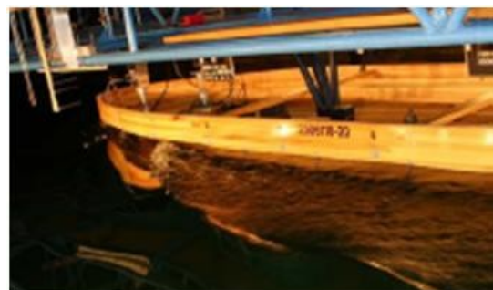
Figure 10: Wave system from FWD thruster head box
