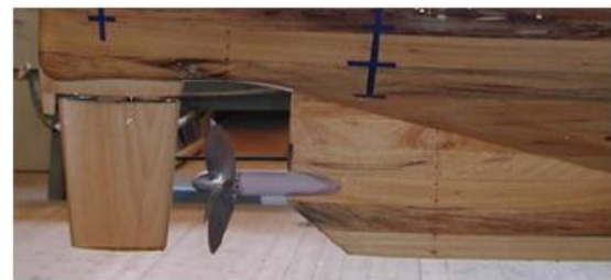
Figure 5: Single open propeller arrangement
