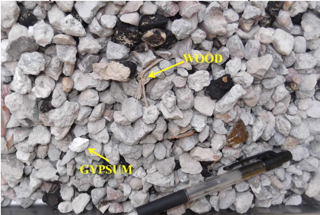
Figure 1 Details of impurities in the 8/16 mm RCA fraction used in this study
