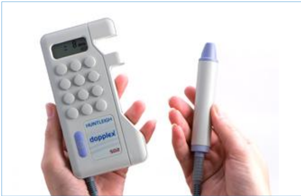
FIGURA 17. Doppler manual portable Dopplex SD2 de 8 MHz (Huntleigh Healthcare Ltd. Cardiff, UK)
