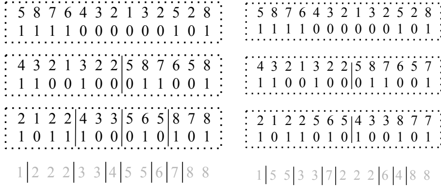
Figure 4.2: On the left, the pointerless wavelet tree (WTNP) of Figure 2.7.1. On the right, the wavelet matrix (WM) over the same sequence. One vertical line per level represents the position stored in the z_\ell values.
