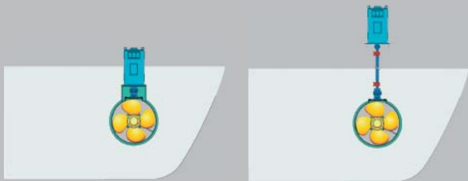
Vertical prime mover directly coupled to the input.
