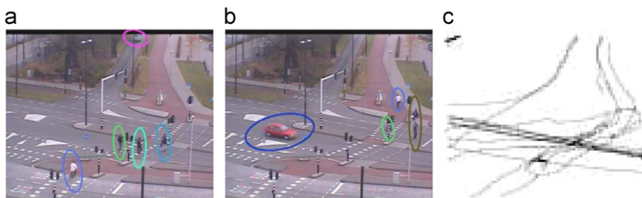
Fig. 4. Online potential example. (a, b) For each target detected, its path is added to the potential image (c). In black, most visited pixels. In white, forbidden positions.
