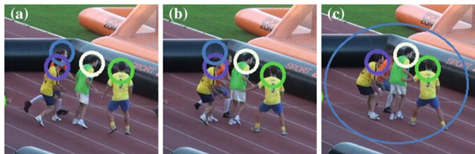
Fig. 14 Ocluded target search example. When the blue target is lost because of bad accuracy (b), the algorithm detects the blob in which the target could reappear (c) (color figure online)
