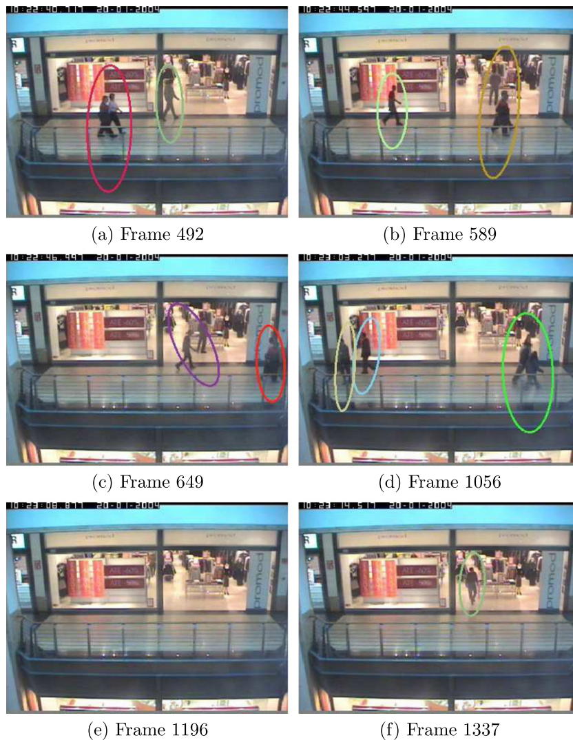
Fig. 18. CAVIAR dataset example. The system can detect both grouping and splitting events, and also long-time occlusions.
