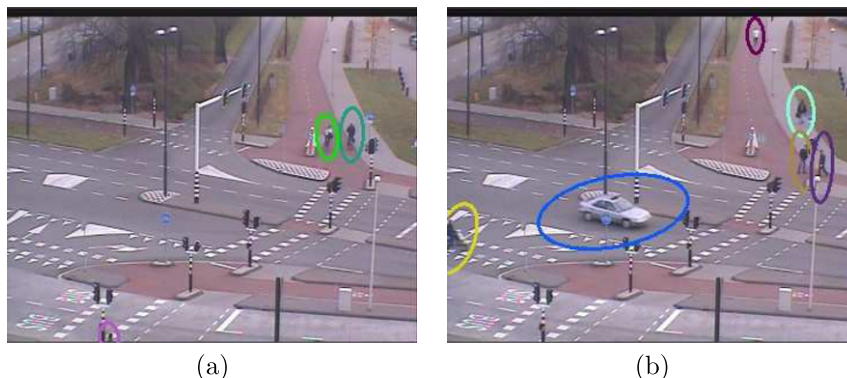
Fig. 6. Low level tracking example using ellipse centroid metric. Each ellipse has a unique color which is used as object id. (For interpretation of the references to color in this figure legend, the reader is referred to the web version of this article.)
