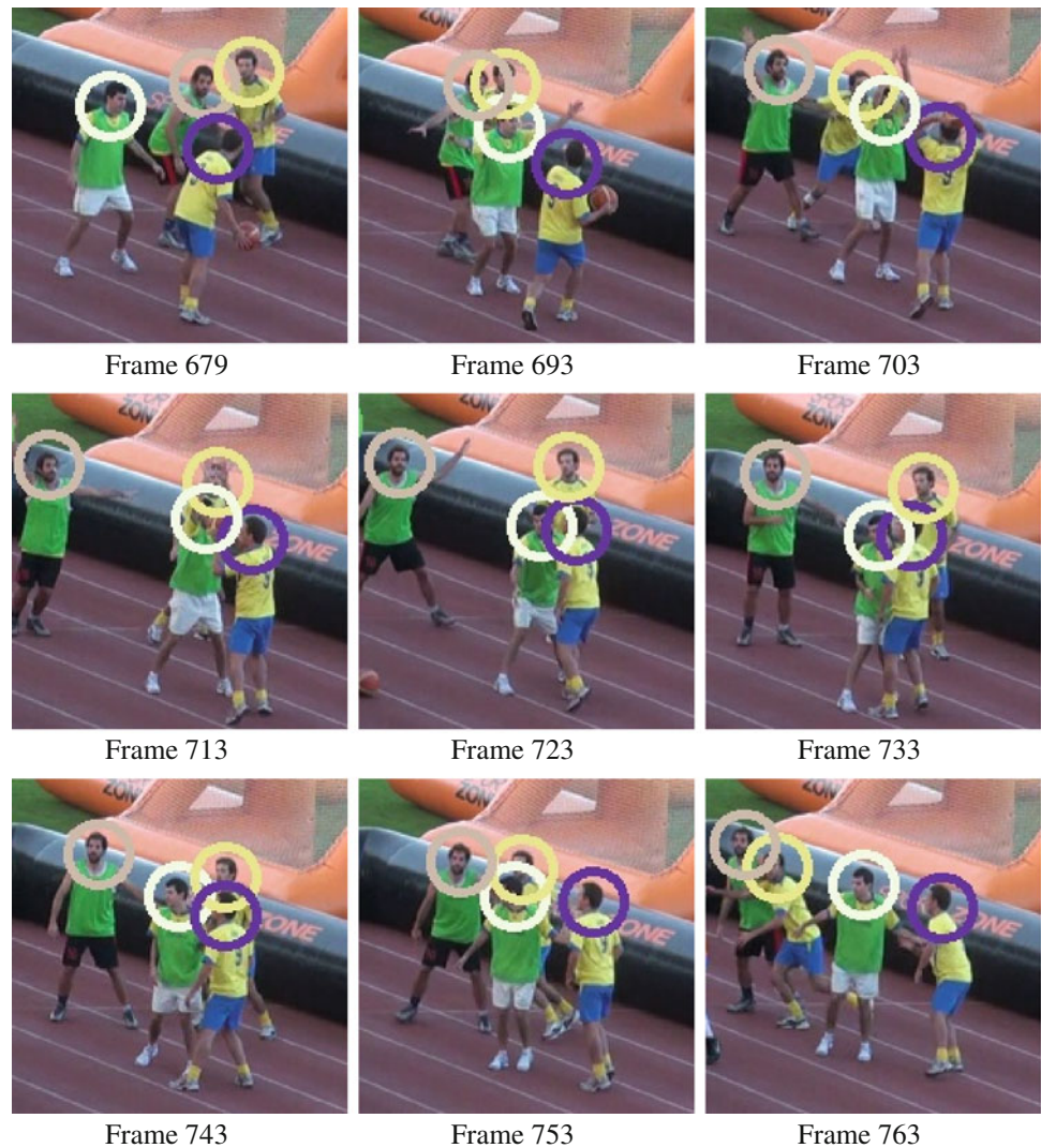
Fig. 18 People detection in crowded scenes. Partial occlusions are solved without using color information. Particle filter system is robust under these situations
