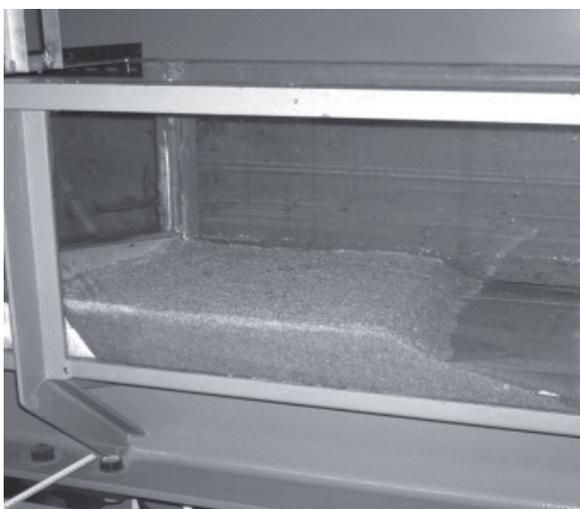
Figure 8. Neyrpic weir with 1 mm sand simulating a broad-crested weir
