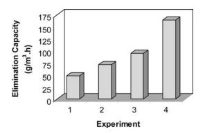
Maximum toluene elimination capacities under different conditions of RH and pH: (1) 85 % RH, pH 4.5, (2) 85 % RH, pH 5.9, (3) 85 % RH, pH 7.5, (4) 100 % RH, pH 7.5
