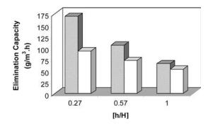
Local elimination capacities in different zones of the biofilters around the end of the experiments, after 4 months operation, for E. oligosperma (left column) and Paecilomyces variotii (right column), showing that toluene removal was more significant near the inlet (h/H=0) than near the outlet (h/H=1) of the reactor
