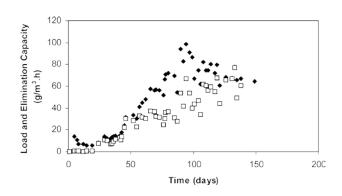
Toluene load (•) and corresponding elimination capacity ( $\Box$ ) versus time in the biofilter inoculated with the black yeast E. oligosperma (85% RH, pH 5.9)
