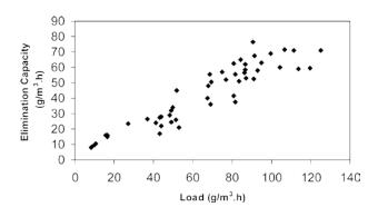
Toluene elimination capacity versus load in the biofilter inoculated with the bacterial-fungal consortium
