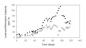
Toluene load (•) and corresponding elimination capacity ( $\Box$ ) versus time in the biofilter inoculated with the fungus P. variotii (85% RH, pH 5.9)
