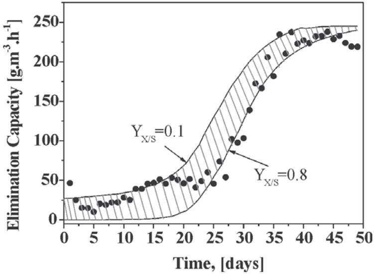
Figure 2. Experimental EC and model simulation. (•) Experimental results and (–) simulation. Variation of the EC simulation for a range of cellular yield in *F. solani* between 0.1 and 0.8 g<sup>-1</sup>g<sup>-1</sup>.
