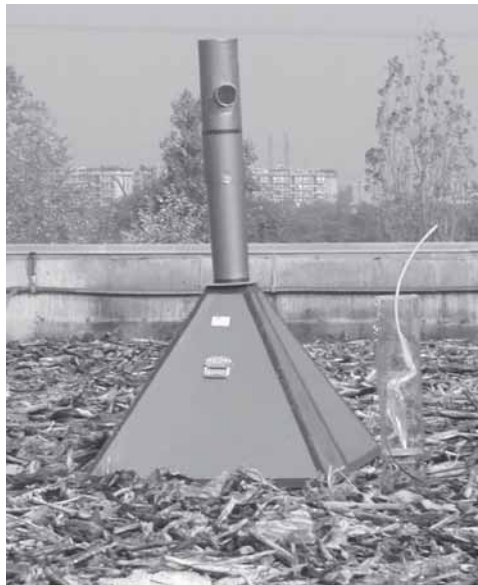
Figure 1. Equipment for odour sampling at a biofilter outlet.
