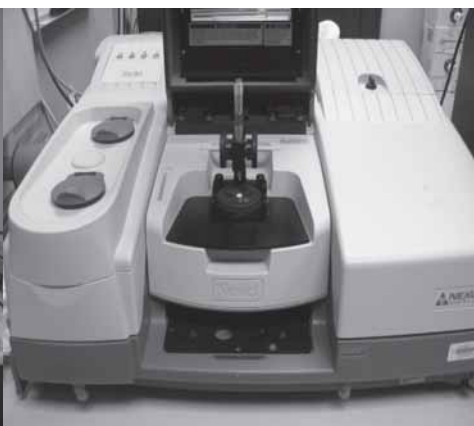
Figure 2. FT-IR bench with Smart Miracle Accessory
