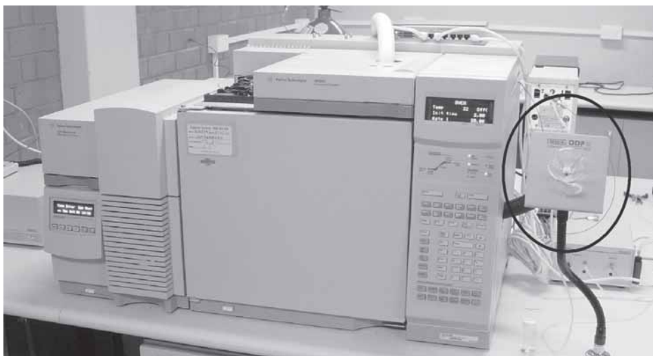
Figure 3. Olfactory-GC-MS showing odour detection port (ODP) on right.
