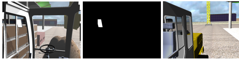
Figure 5.5: Pictures corresponding to the main view, the stencil mask and the mirror view.
