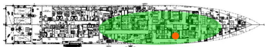
FIGURE 15. Blueprint of the OPV showing the active UHF RFID coverage (horizontal projection).
