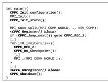
Fig. 1: CPPC instrumentation for stop-and-restart fault-tolerant applications.
