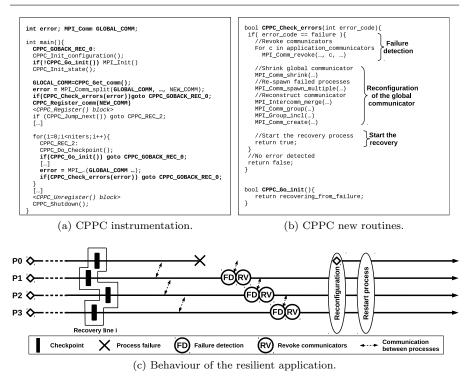
Fig. 2: Resilient MPI applications combining CPPC and ULFM.
