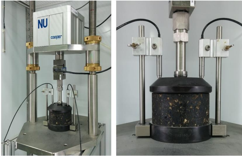
Figure 3. Arrangement of repeated load axial test according to Standard BSi DD 226:1996 (BSi, 1996)
