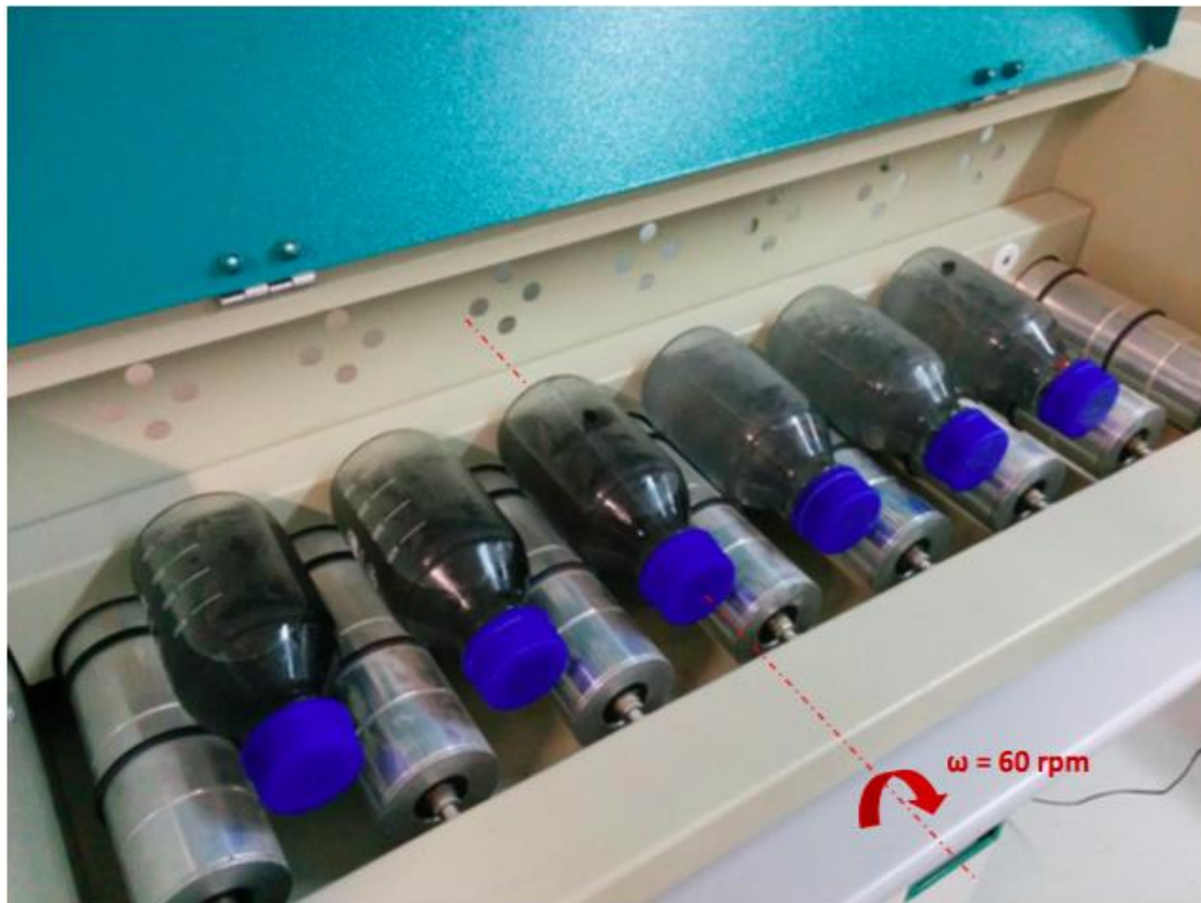
Figure 2. Arrangement of two different samples (6 subsamples) during the rolling bottle test
