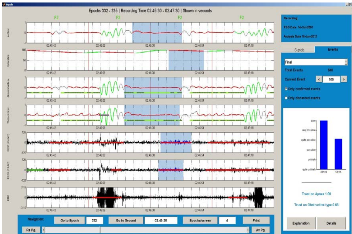
Figure 5.54. Signals visualization interface in which an event is selected for visualization. Integrating events composing the full diagnostic pattern are marked in blue. Summary information on event's characterization can be shown on the right bottom area of the window
