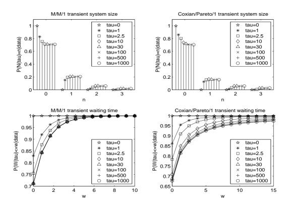
Figure 7: Transient distributions for queue length (top) and waiting time (bottom) for the M/M/1 and Coxian/Pareto/1 systems. These approximate the stationary distribution as  $\tau$  increases. The speed of convergence of the transient waiting time is slower for the Coxian/Pareto/1 than for the M/M/1 system.
