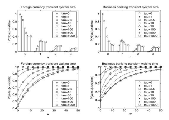
Figure 10: Predictive transient queue length (top) and waiting time (down) distributions for the bank systems. These approximate the stationary distributions as  $\tau$  increases but the speed of convergence is slow. For the business banking system, there are still differences between the waiting time distributions after 500 and 1000 minutes.
