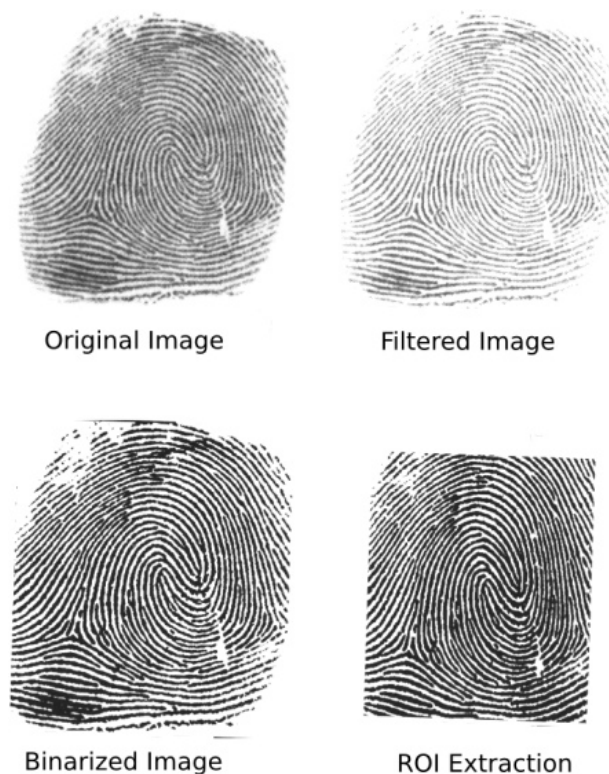
Figure 1.9: Result of applying consecutively different techniques to the fingerprint image prior to the feature extraction.
