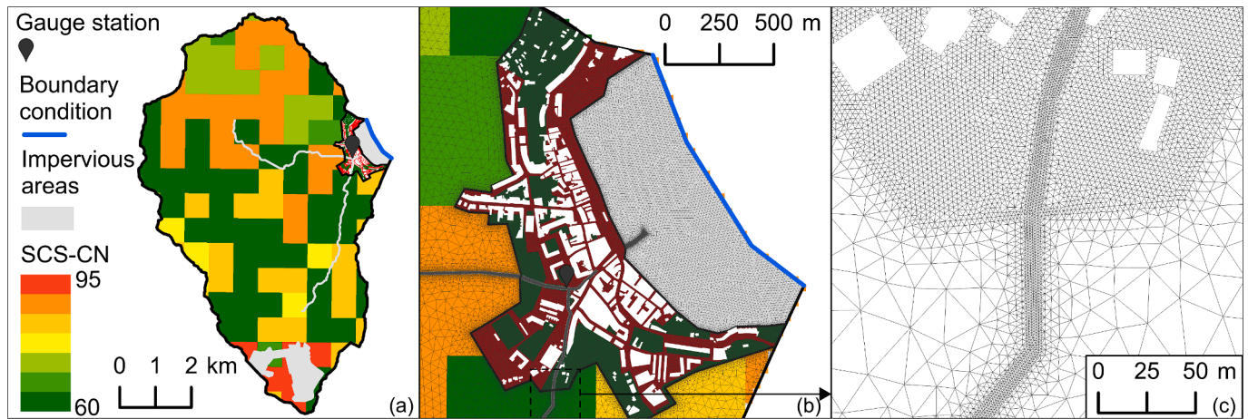
Fig. 3. SCS-CN values in the whole catchment (a), SCS-CN values in the study area (b), and detail of the numerical grid within the study area (c).
