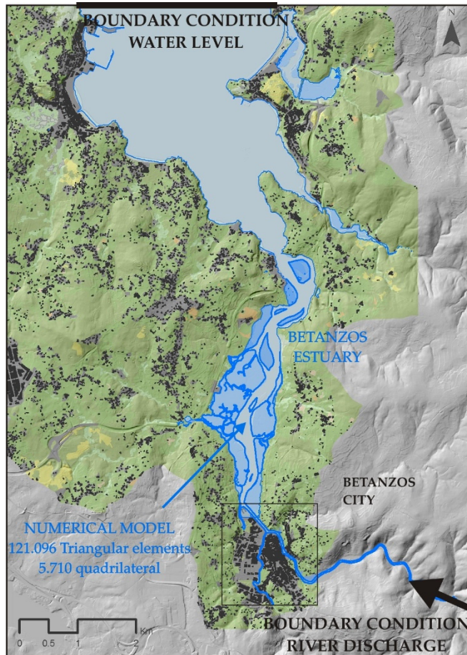
Figure 2. Spatial domain of the numerical simulations and location of the open boundaries.
