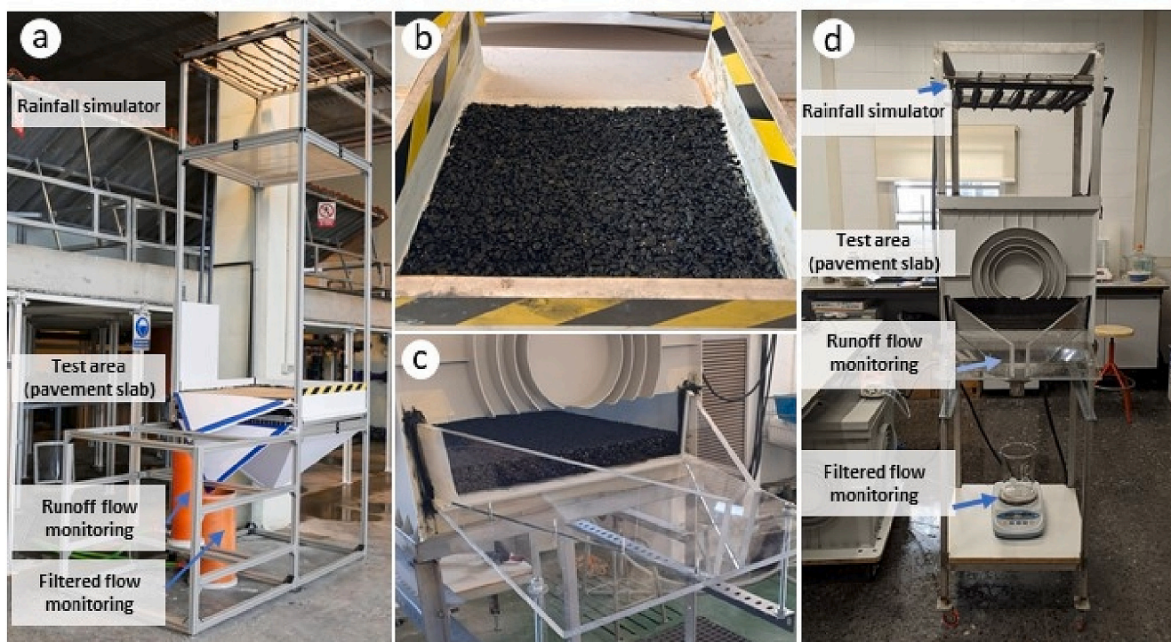
Fig. 1. General views of the UDC (a) and UPV experimental setup (d). Detail of the asphalt slab installed in the test area of each rainfall simulator and including the runoff collection system (b and c, respectively).
