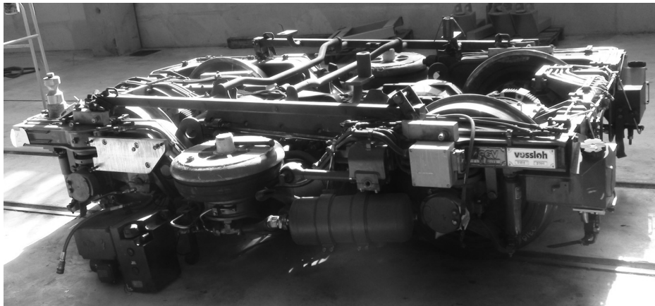
FIGURE 5 Alicante vehicles trucks: a) Bombardier light rail; b) Vossloh tram-train.
