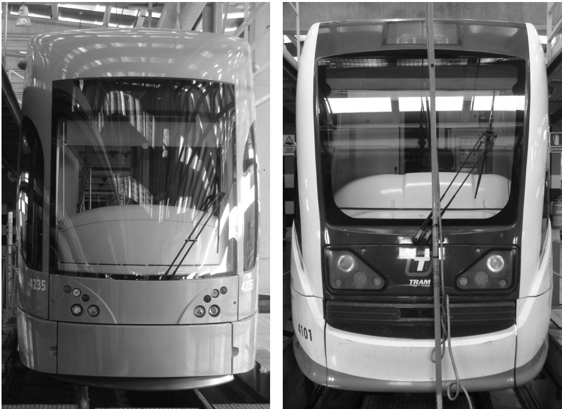
FIGURE 8 Exterior lights of Alicante vehicles: a) Bombardier light rail; b) Vossloh tram-train.
