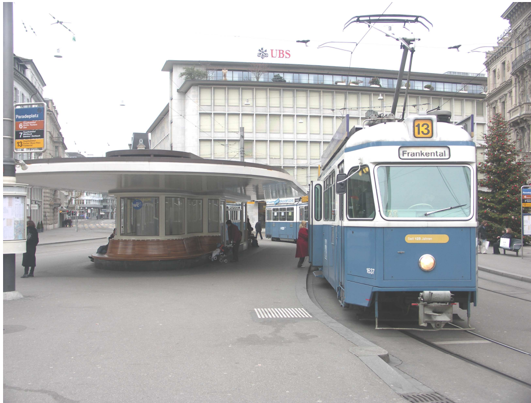
FIGURE 4 Effects of horizontal curves at stations. Zurich (Switzerland) light rail.
