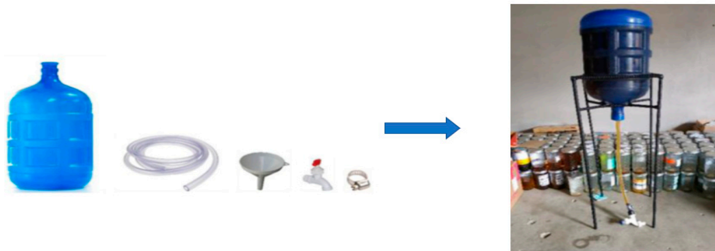
Figure 4. Used materials for the fabrication of the artisanal decanter.
