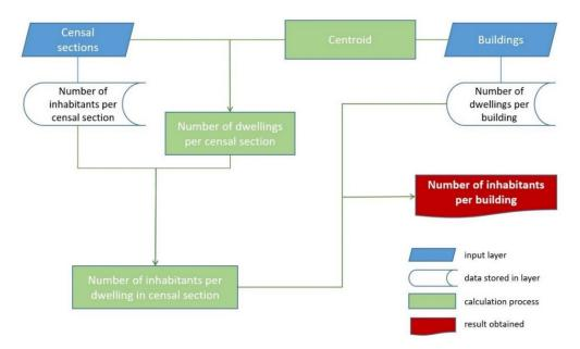
**Figure 3.** Flowchart of the procedure for estimating the number of inhabitants per building from data based on census sections.
