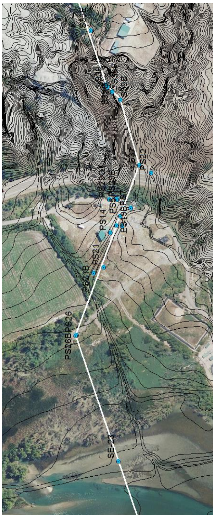
Figure 4.2. Map of the site with the outline of the E-W hydrogeological profile and the location of the boreholes along the profile.
