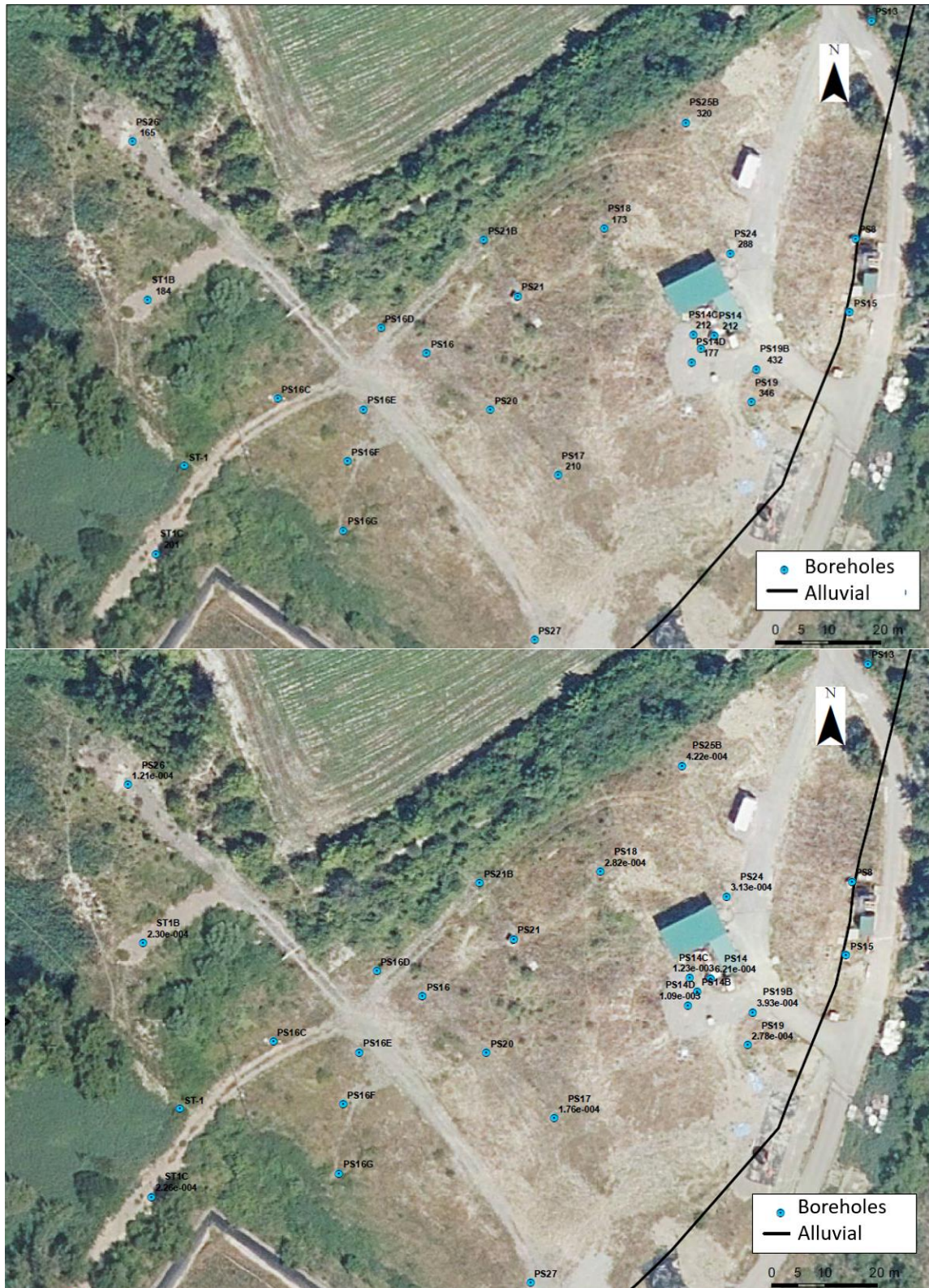
Figure 9.6. Values of hydraulic conductivity, K, in m/d (upper figure) and specific storage coefficient (m -1 ) estimated by Suso (2018) from the interpretation of the drawdowns with the Theis method.
