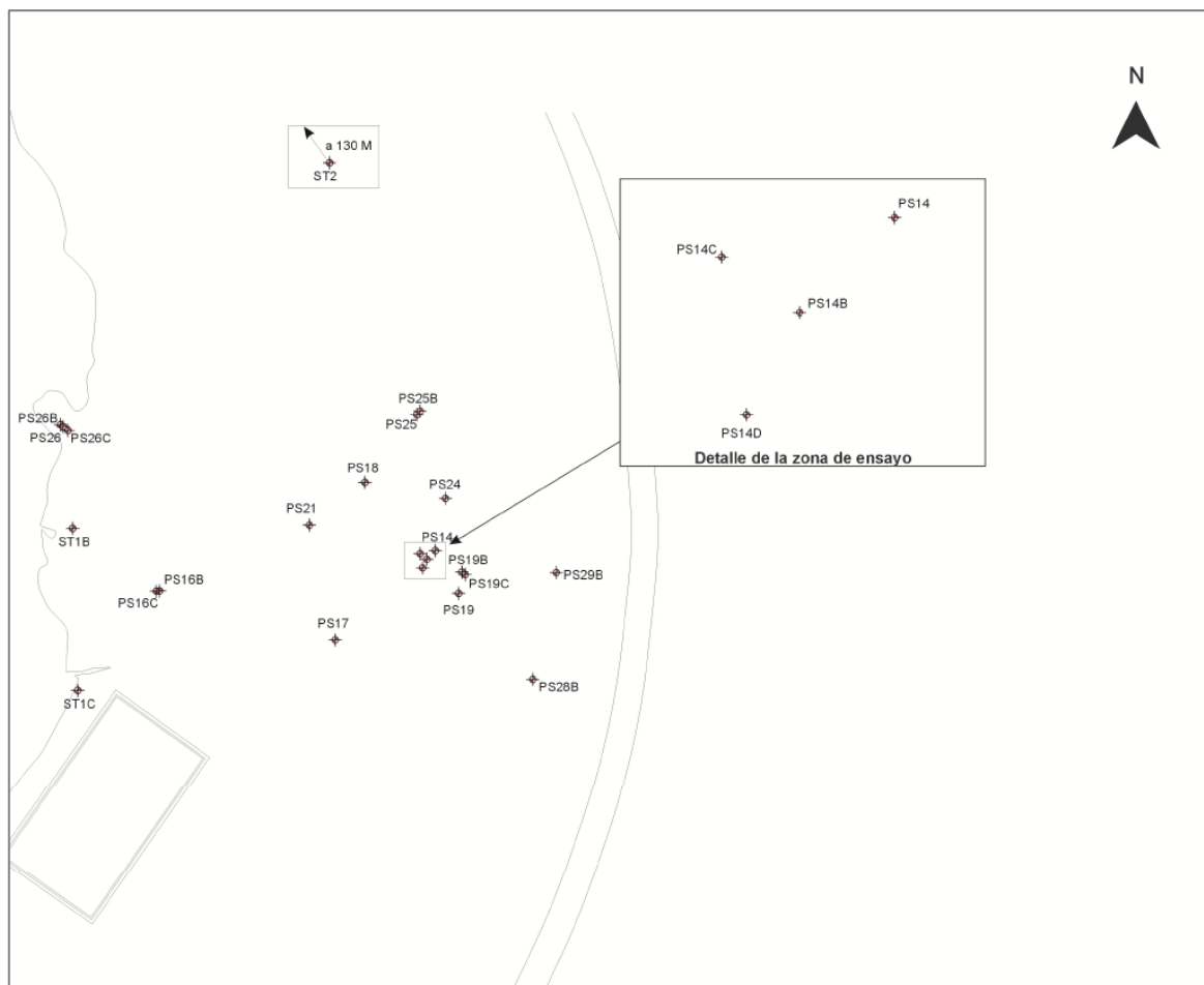
Figure 10.1. Location of the observation and injection boreholes in the tracer test area (EMGRISA 2018).
