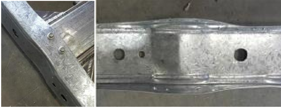
Figura 62. Detalle de la deformación de la viga carril. Ensayo experimental. (Fuente: [2] “Lateral performance of a new hybrid CFS shear wall panel for mid-rise construction”)
