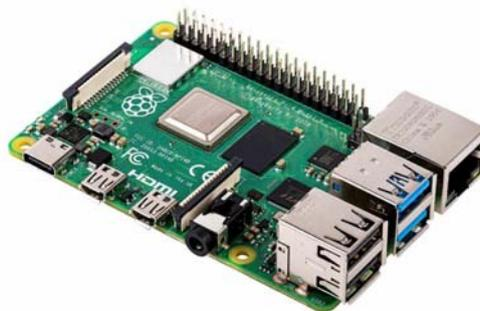
**Figura 7.15** – Raspberry Pi 4 Model B [39].
