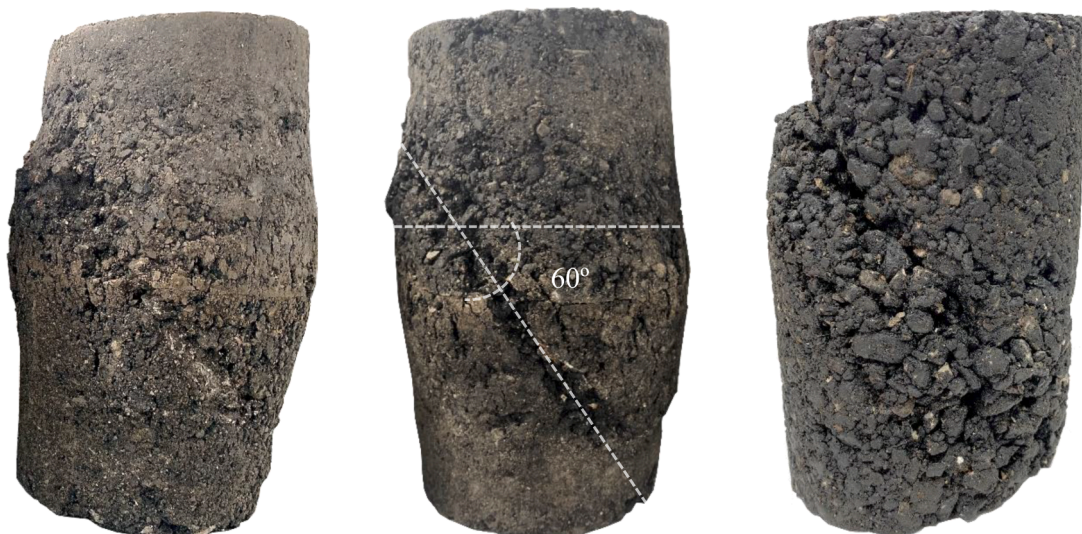
Fig. 9. Shape of CIR specimens after monotonic triaxial test. Failure plane at approximately 60°.
