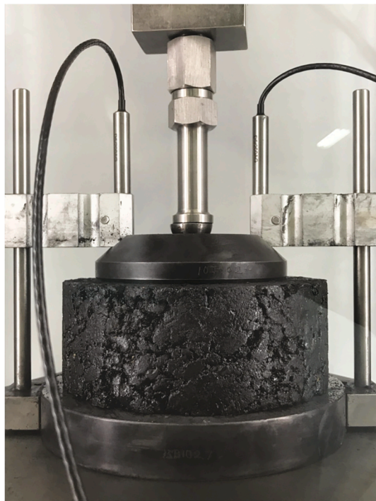
Fig. 7. Confined uniaxial cyclic compression test.
