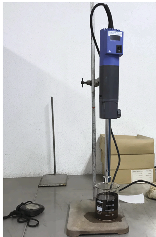
Fig. 3. Blend of bitumen emulsion with byproduct using ultra turrax.
