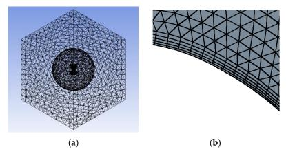
Figure 4. (a) Computational mesh; (b) boundary layer detail.
