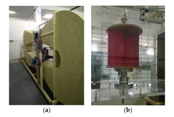
Figure 6. (a) Wind tunnel used for the measurements; (b) turbine inside the test section.
