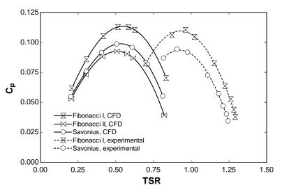
Figure 7. Power coefficients against TSR for Fibonacci I, Fibonacci II, and Savonius configurations.
