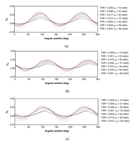
Figure 8. Power coefficient against the angular position; (a) Fibonacci I; (b) Fibonacci II; (c) Savonius.
