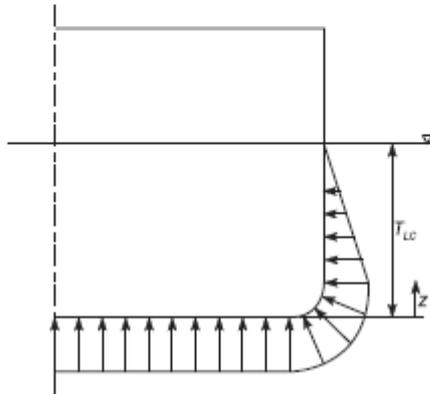
**Figure 1 Transverse distribution of hydrostatic pressure  $P_S$**
