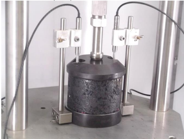
5 6 7 FIGURE 4 repeated-load axial test device.
