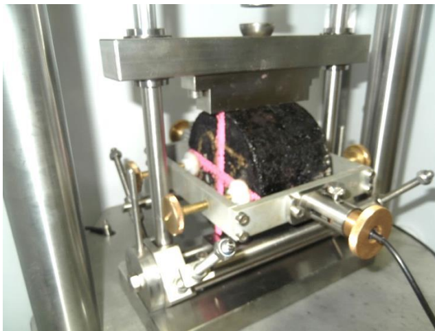
24 FIGURE 3 indirect tensile stiffness modulus test device.
