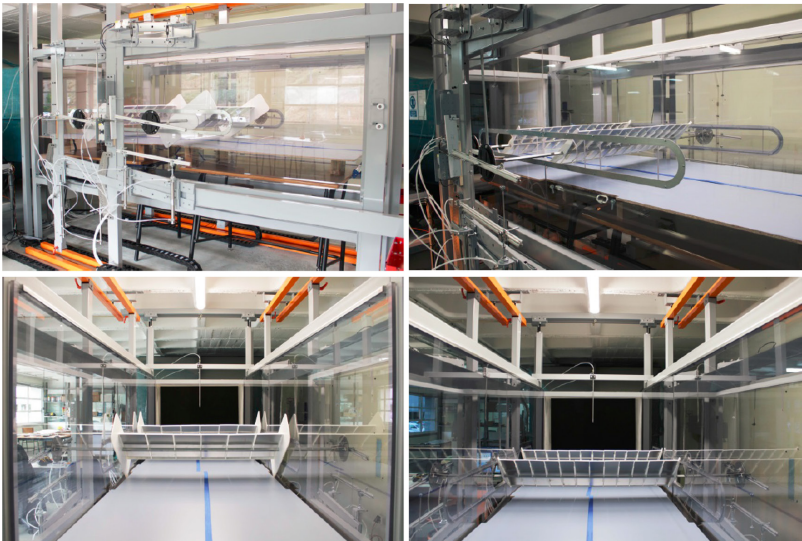
Figure 11: Wake setup of the solar tracker for configuration 1 (left) and configuration 2 (right).
