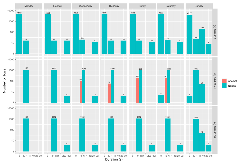
Figure 10. Log-linear flow duration. (a) Broker. (b) An abnormal node. (c) A normal node.
