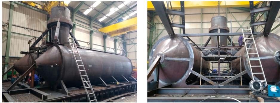
Figure 3. Building of the BlueSATH ® platform in the workshops. Source: Figure courtesy of Saitec [31].
