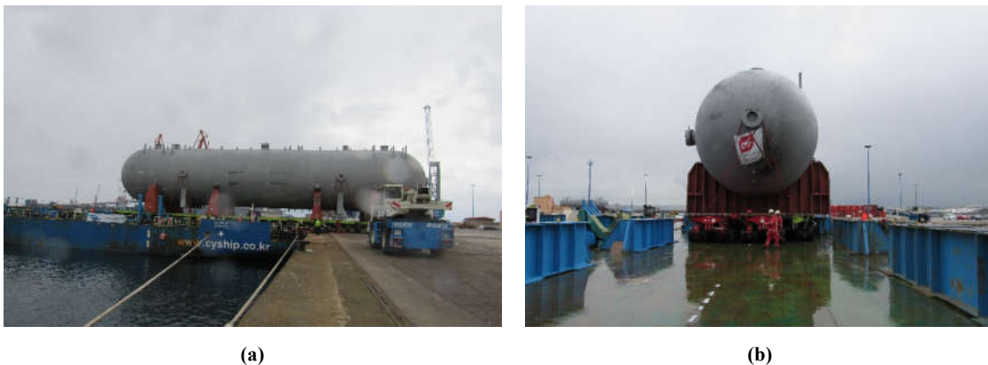
Figure 2. (a) Loading operation by a self-propelled modular transporter (SPMT); (b) GSC cradles passing over the grillage beams until they reach the stowage position.
