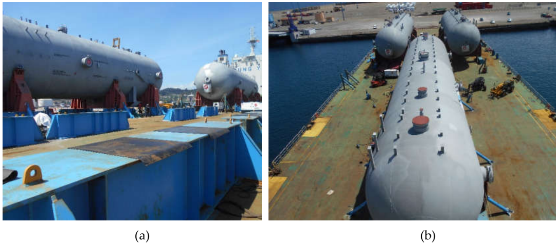
Figure 6. (a) Rubber mats above the grillage beams in the GSC's footprint area. (b) Shipment's final stowage.
