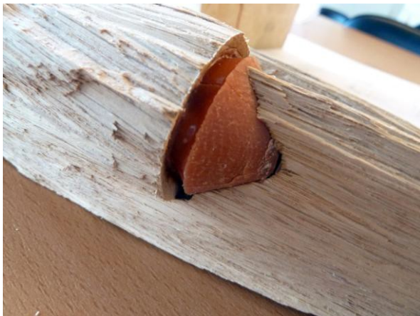
Figure 5: Adhesive bulbs to improve the axial strength of steel threaded bars glued in timber
