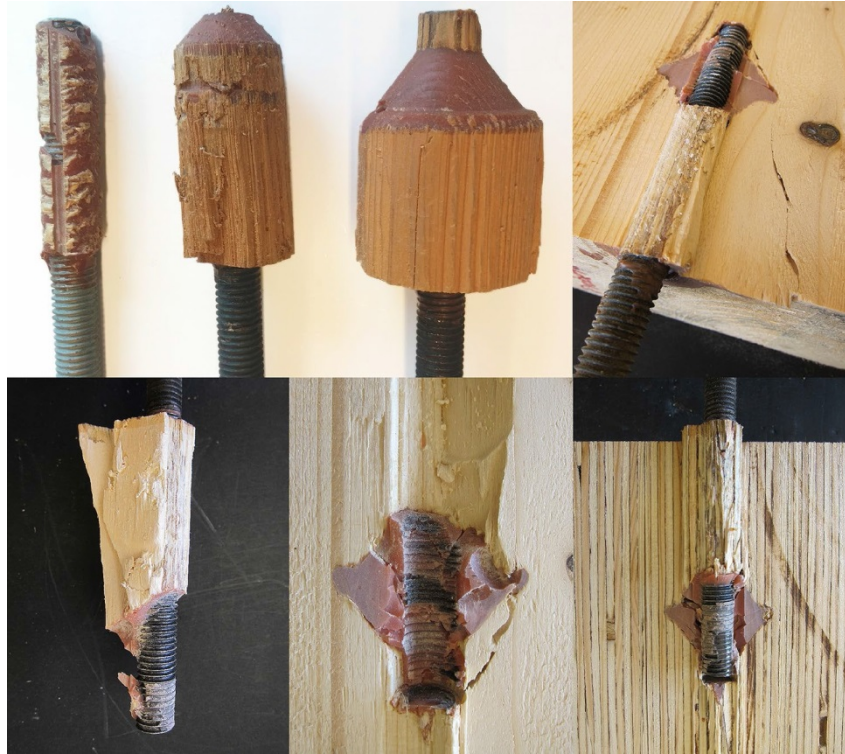
Fig. 9 Top: extraction of the bulb, dragging out a block of timber, the predominant failure mode in test pieces with shorter anchorages. Bottom: breakage of the adhesive bulb, the predominant failure mode in test pieces with medium length anchorages
