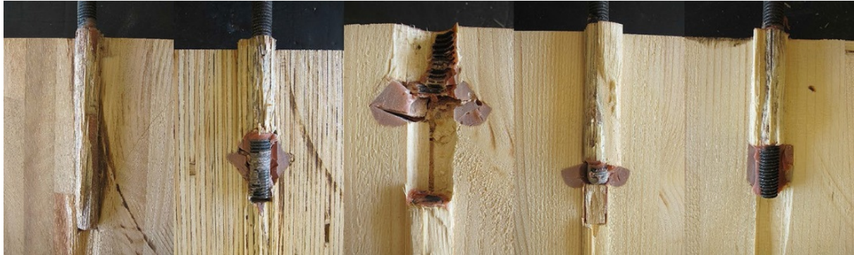
Fig. 7 Cylindrical anchorage (type 0—Fig. 4) and different configurations of bulbs, which were tested (type IIa, IIb, IIc and IIc in Fig. 4, respectively)
