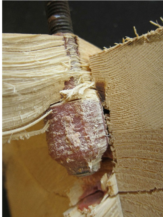
Fig. 11 Extraction of the bulb and crushing of the wood, the predominant failure mode in test pieces with an anchorage perpendicular to the fibre
