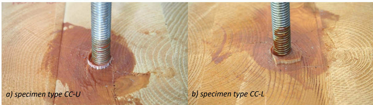
Fig.5. Failure mode presented by all the tested specimen after testing them until failure. Shear failure on timber/adhesive interface.
