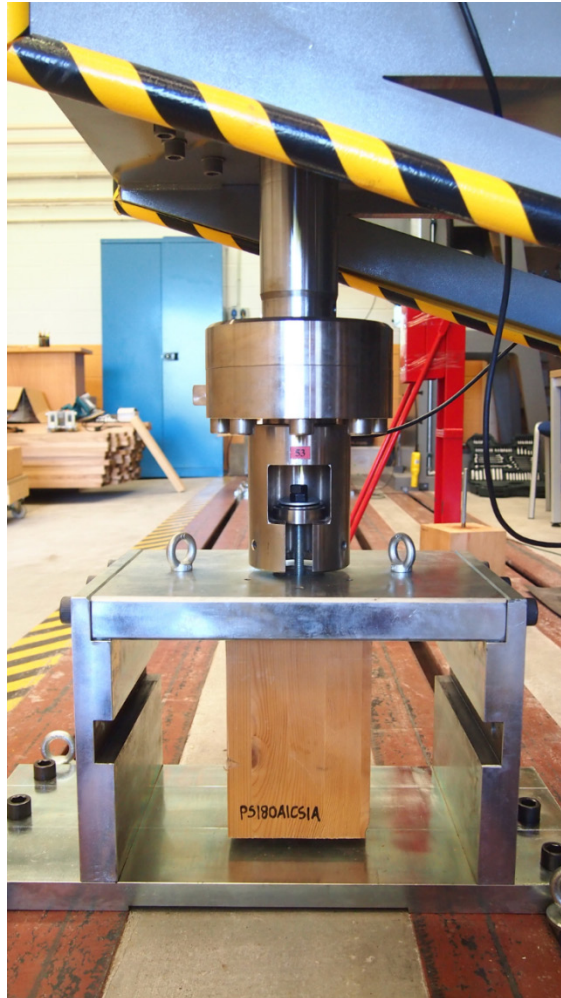
Fig. 1. Pull-compression test device.
