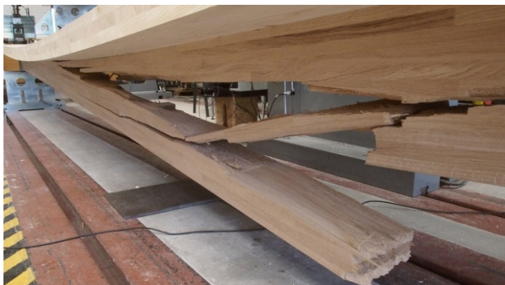
Fig. 11. Failure close to a finger joint in the specimen F1/OAK-3.
