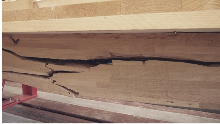
Fig. 12. Bending failure in a pretensioned T-section corresponding to specimen F2/OAK-3.
