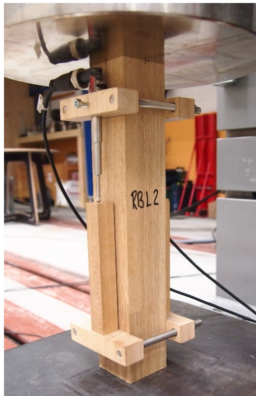
Fig. 5. Test to determine the compression MOE parallel to the grain.
