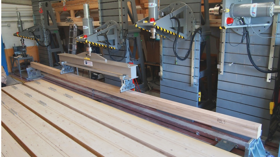
Fig. 4. Bending test to determine the global bending MOE.
