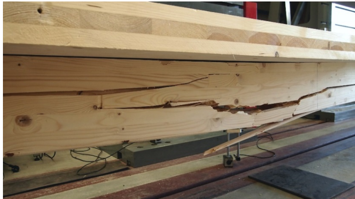
Fig. 9. Typical bending failure in non-pretensioned T-sections corresponding to specimen F1/PIC-1.
