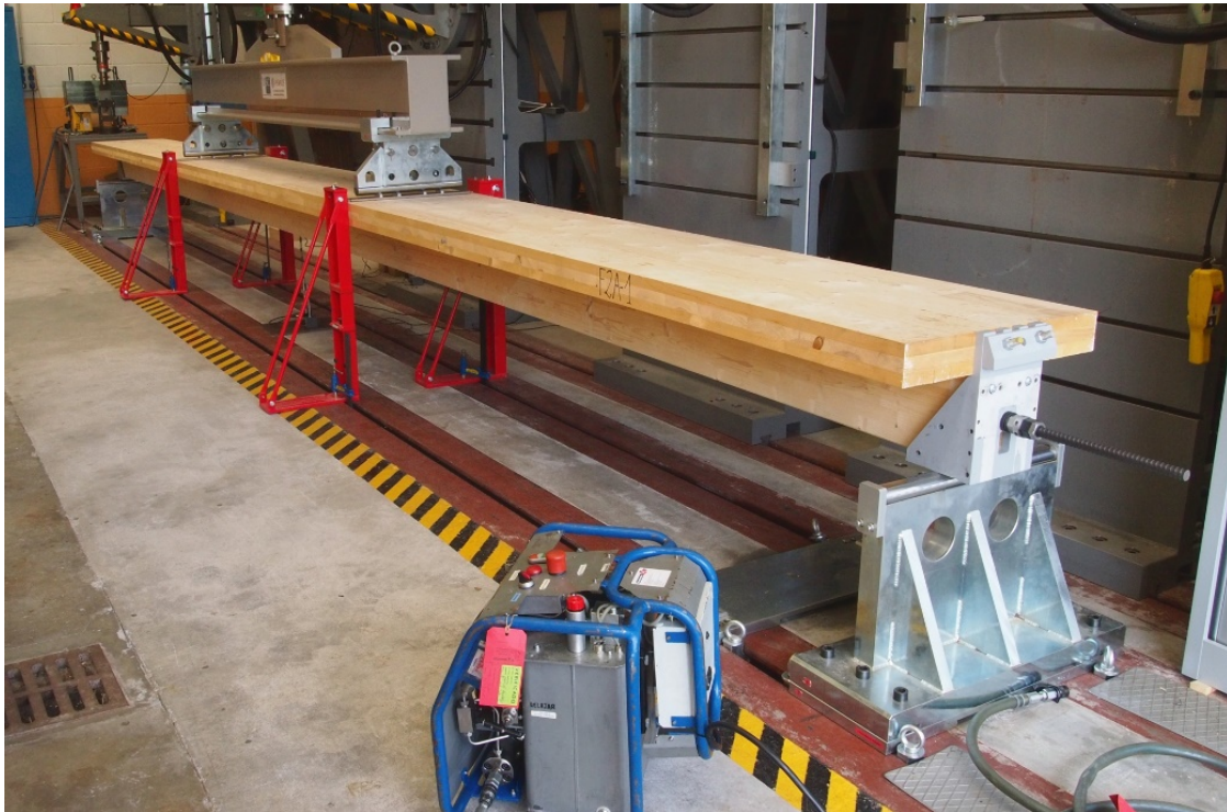
Fig. 6. Test of a pretensioned T-section with Picea abies webs.
