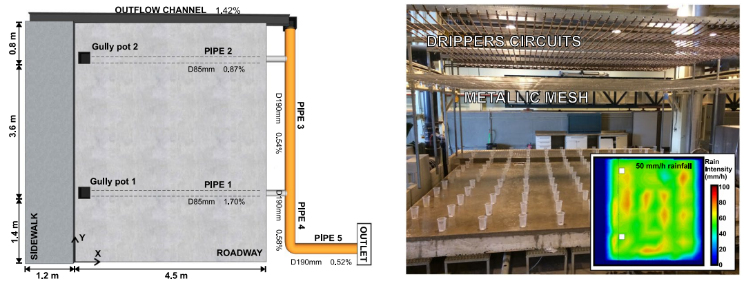
Fig. 1 Street section physical model scheme and general image of the rainfall simulator with the experimental setup for the measurement of rain intensity maps. Results for the intermediate rainfall are also plotted.
