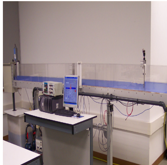
Figure 1: Prototype hydraulic canal in laboratory
